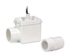
Automatically detects clogged A/C condensate drains and shuts off the system for enhanced safety protection. Installed horizontally on the auxiliary drain outlet of the primary pan, using the provided adapter, bushing, and cap. Cap can be easily removable for inspecting the operation of float switches.
