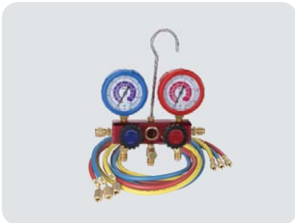
Testing manifold set for R404a,R407a,R134a and R22 manifold with 3pcs house, 2pcs qc12 quick couplers and 2pcs 2-3/4"dia.guage, 1/4"seaconnection. 3pcs 36"house.3pcs 60"house.3pcs 72"house.all house are desinged for working pressure 800psi bursting pressure 4000psi
